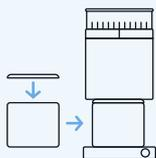
Place the catch lid on the catch and slide it beneath the chute.
